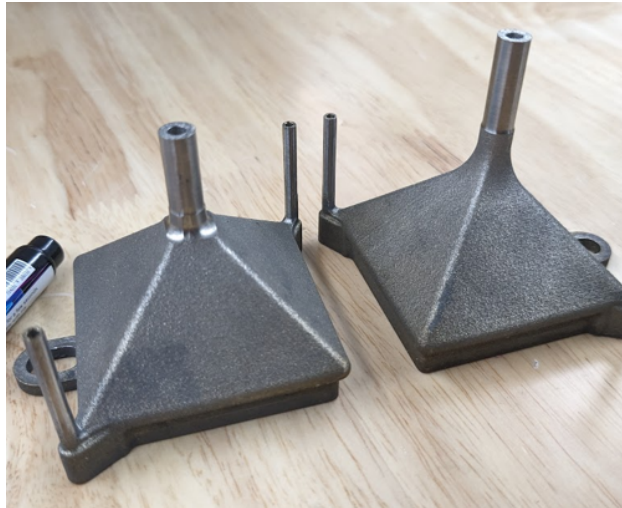
Figure 7: Two Manufactured Evaporators
