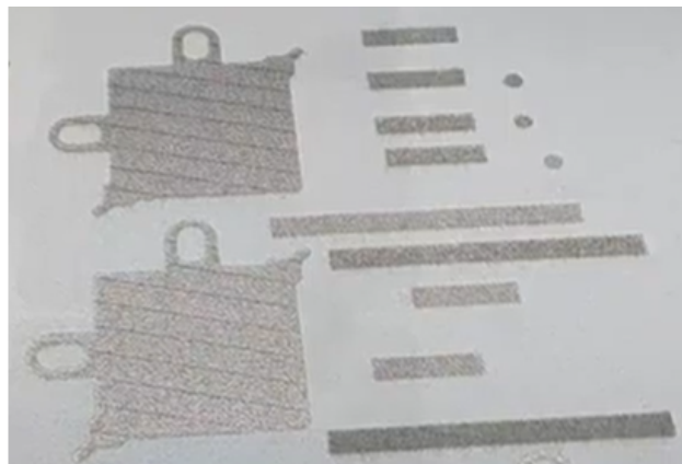
Figure 6: An in-process additive manufacturing run, showing 2 evaporator samples, as well as test coupons to verify print porosity and permeability (short rectangles), pore size (long rectangles), and electrical and thermal conductivity (small circles)
